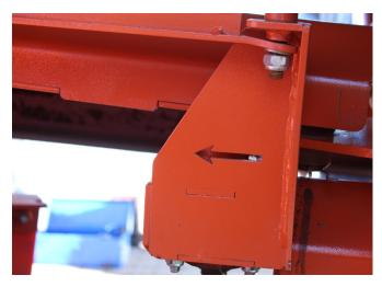
STEP 11: The bolts securing the sliding arms of the tracker must now be loosened to allow the tracker to be centered, the tracker must sit in the middle of the stringers and not the belt.
