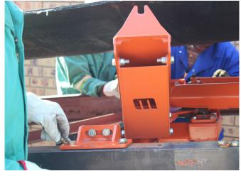
STEP 12: The distance indicated should be the same on both sides of the unit. Once this has been done the bolts on the sliding arm as in Step 11 must be tightened.
