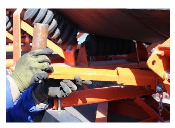
STEP 16: Measure the height difference between the top of the center idler and the belt. Remember that the tracker should be elevated between 10mm and 25mm above the surrounding idlers to ensure correct operation and grip. Take the difference measured and add the 10mm. This measurement is how much the unit is to be raised.
