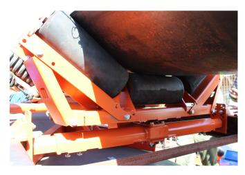
STEP 19: The wing rollers can now be raised to the correct position and adjusted. The rollers should both be approximately 10mm from the belt edge. Once this has been done tighten the bolts and nuts.
