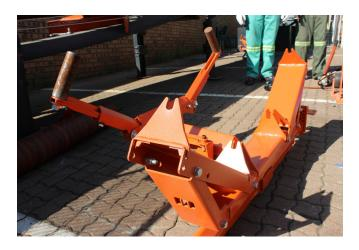
STEP 2: Remove wing roller arms and one idler side bracket to allow easier installation. This will allow the unit to be pushed under the belt from the side.
