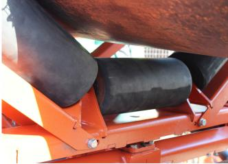
STEP 17: The calculation from above is the amount by which the unit is to be raised. Mark the correct bolt hole on the arm and raise accordingly. Insert the bolts and nuts and tighten.
